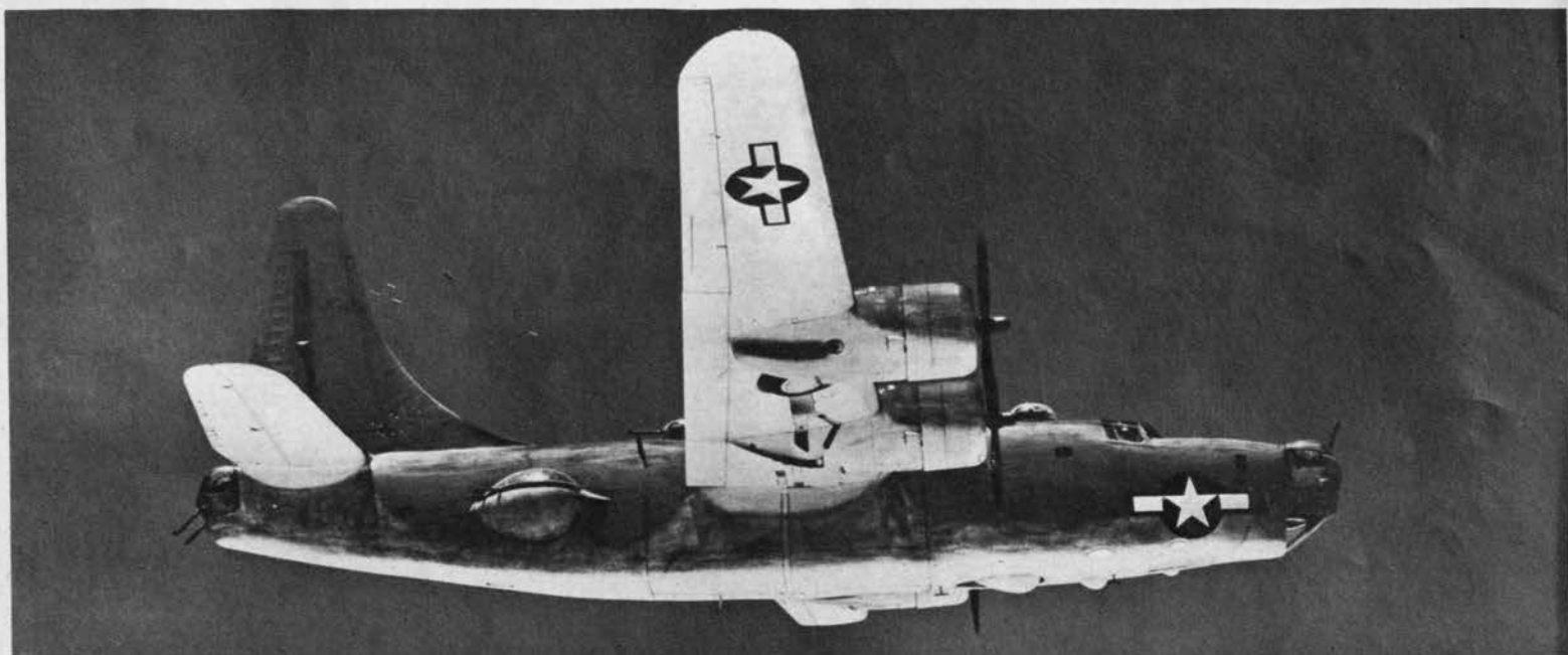
PB4Y-2'S CENTERED WING, LONG NOSE, LARGE SIDE TURRETS AND TWO TURRETS ATOP FUSELAGE DISTINGUISH IT FROM EARLIER LIBERATOR MODELS
